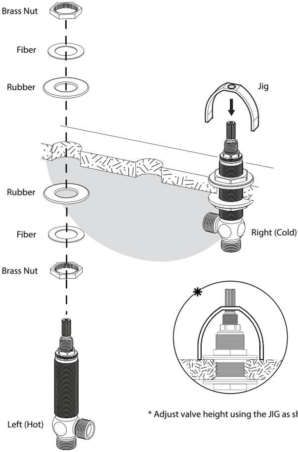
\* Adjust valve height using the JIG as shown
